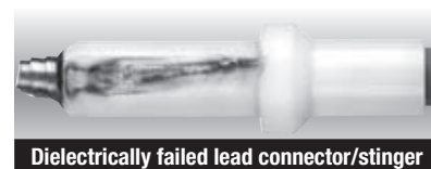
Dielectrically failed lead connector/stinger
